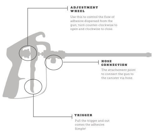
The Bead Gun has been developed for use in conjunction with Polyurethane Foam Insulation adhesives like QD3000. The Bead Gun is not suitable for use with any web spray contact adhesives, primers or fleeceback adhesives.
